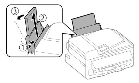
2. Raise the paper support and its extension, pull out the output tray, then raise the paper stopper.
